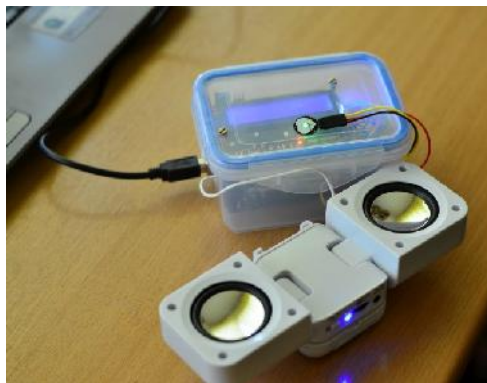
Figure 4: The experimental device with pulse sensor and sound shield.
