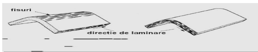
Figure 7: Bending transverse direction producing crackers.
