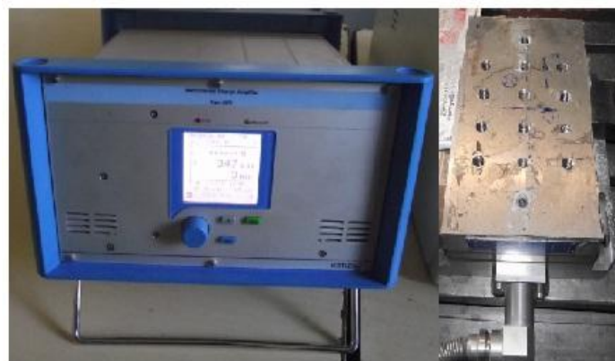
Figure 3: Kistler torque measurement construction [6]
