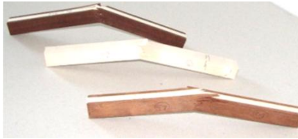
Figure 3: The samples after bending fracture
