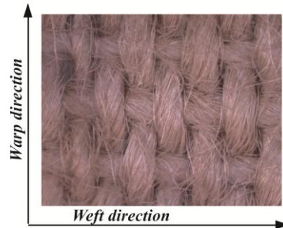
Figure 1: Photos aquired by digital microscope in case of the jute woven fabric used for reinforcing
