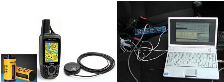
Figure 1. The GPS devices used in measurements (from left to right): Holux M-241; Garmin GPSMap 60CSx; GPS 18x-5Hz; Racelogic VBox (the blue case) and the previous two devices
