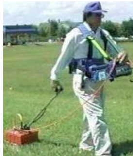
Figure 11: Soil penetration device with radar (after GeoModel, 2007)
