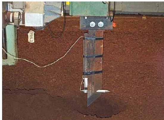
Figure 8: Measuring device of soil resistance in horizontal plane with acoustic sensors
