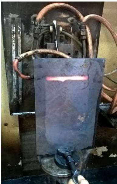
a. CIF process of material in LGS profile
