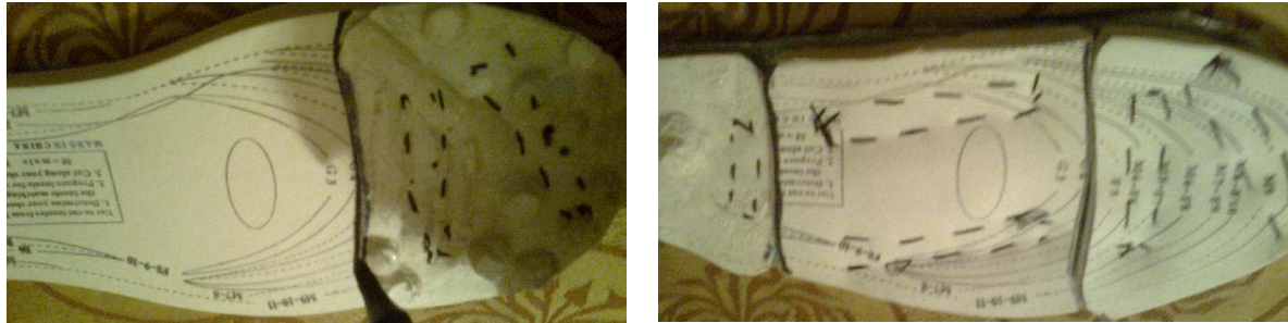
Figure 4: Sponge high density elements disposing on the core silicone items, for wearing comfort increasing
