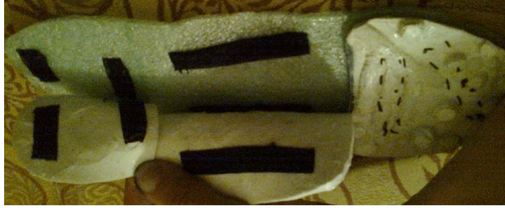
Figure 3: Example of disposing a silicone item (via Velcro elements) to the sponge layer To increase the lifetime and resistance of the foot insole, and to increase the wearing comfort, another sponge layer (high density) was used as base for disposing to each silicone item (Figure 4):
