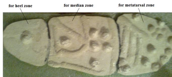
Figure 2: Silicone core dividing into three items specific for each plantar area
