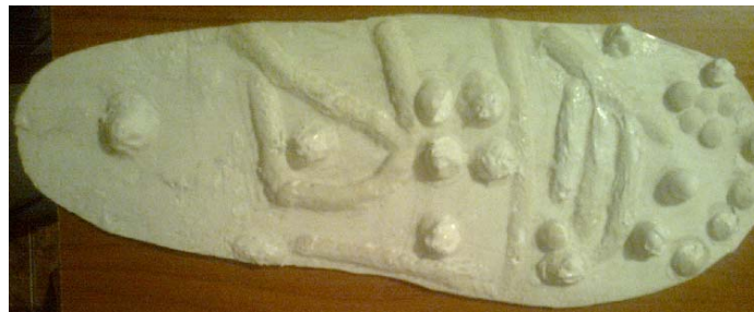
Figure 1: Obtaining the silicone core
