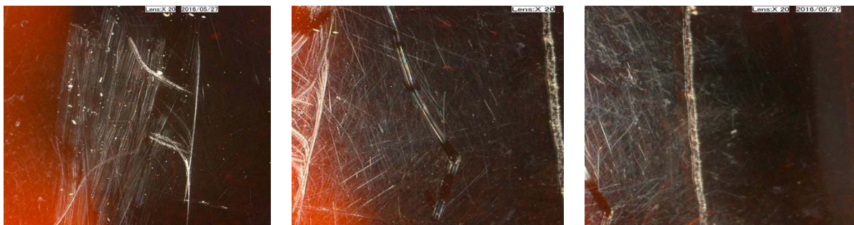
Figure 7: Attempted mechanical aggression controlled by wood (left), metal (middle), stone (right) of the ski goggle lens (digital microscope images with 20x magnification)
