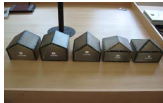
Figure 2: The real greenhouse forms (machetes at 1:20 scale) chosen to study wind loads using the Lattice Boltzmann Method (LBM)
