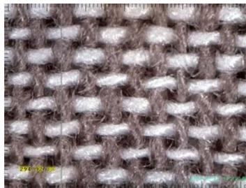
**Figure 1:** Flax woven fabric used as reinforcing material
