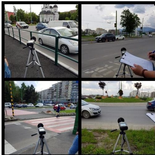
Fig. 3.1. – Use of sound level meter for noise measurement at the intersections studied
