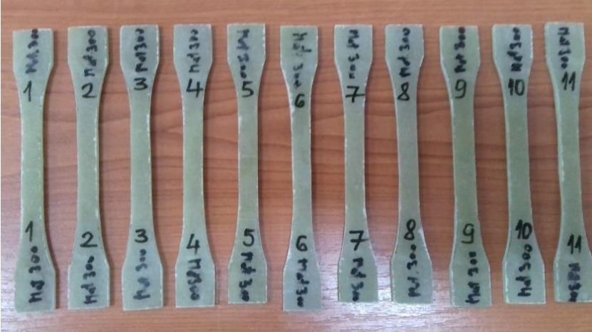
Figure 1: Size and shape of MAT300 specimens (courtesy of Compozite Ltd., Brasov)
