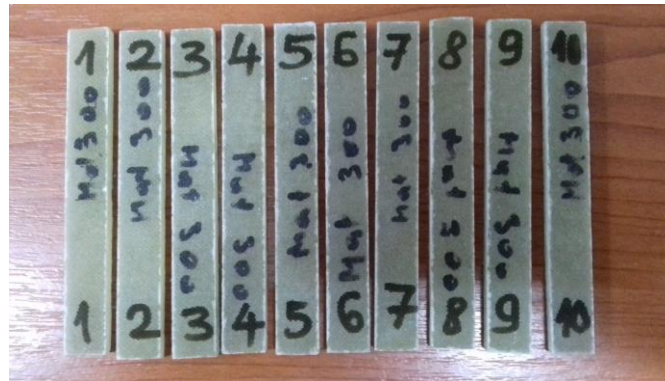
Figure 1: MAT300 specimen's geometric characterization (courtesy of Compozite Ltd., Brasov)
