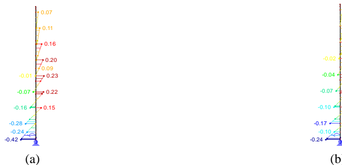
Figure 12: Bending moments at the bottom of the uprights for both rack types: (a) rack type A ( k_{BEC} = 51 kN·m/rad); (b) rack type B ( k_{BEC} = 102 kN·m/rad).
