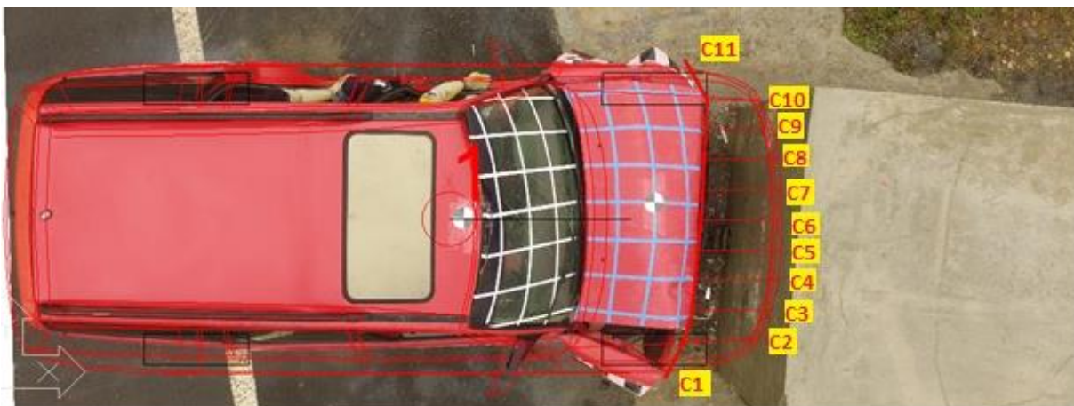
Figure 2: Post-collision vehicle static crush measurements
