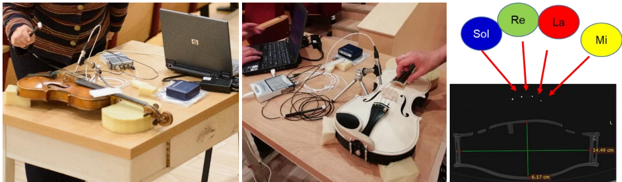
Figure 2 Testing the violins: a) excitation with the impact hammer; b) excitation of the strings of the violins in Pizzicato style; c) the position of the four strings and the musical note corresponding to the tuned free string
