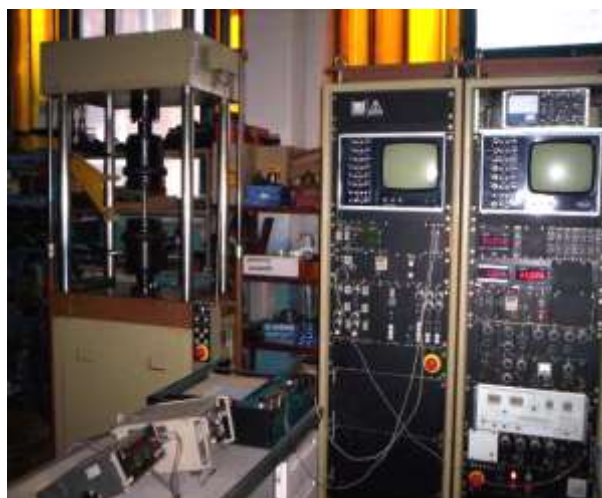
Figure 3. Tensile test stand
