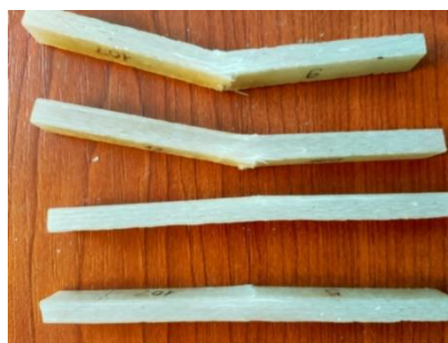
Figure 2. Composite material sample after bending stress
