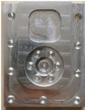
Figure 3: Machining at cutting speed of 500mm/min
