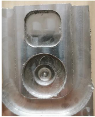
Figure 2: Machining at cutting speed of 500mm/min
