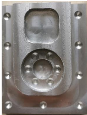
Figure 4: Machining at cutting speed of 150mm/min
