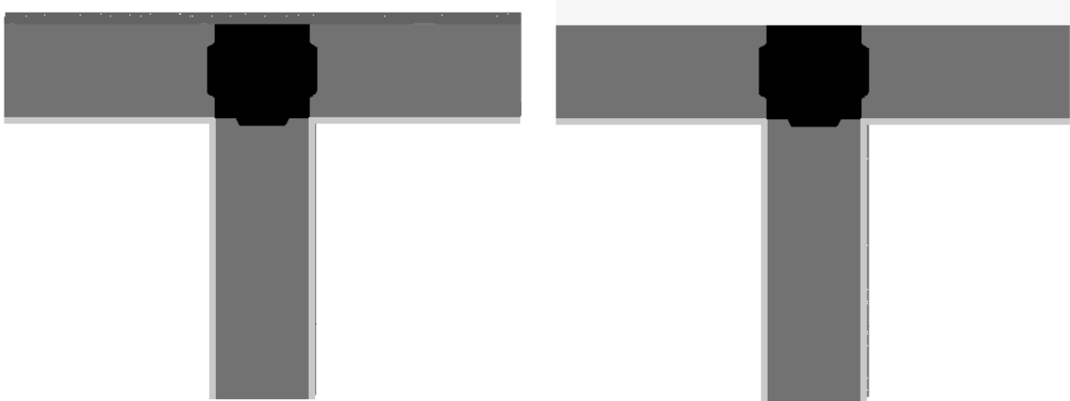
Fig. 12 Geometric modeling of the uninsulated and thermal insulated intersection using the equivalent thermal conductivity of the masonry \lambda_{ech}
