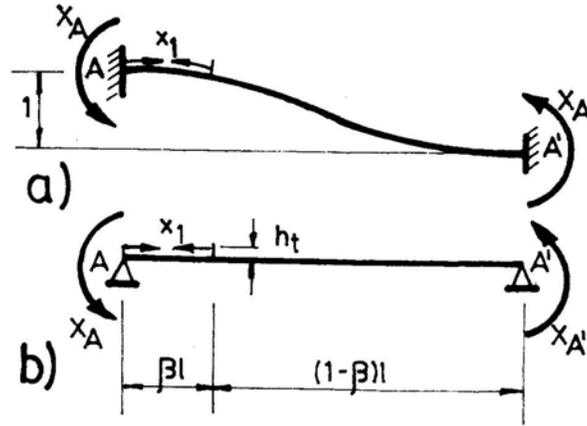
Fig. 4 – Prestressed Bar at One of Its Ends
