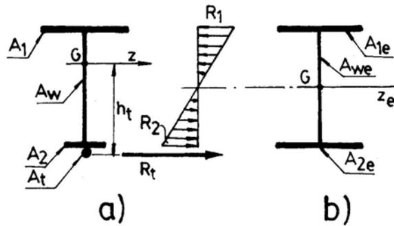
Fig. 2 a). Prestressed Section; b). Equivalent Section
