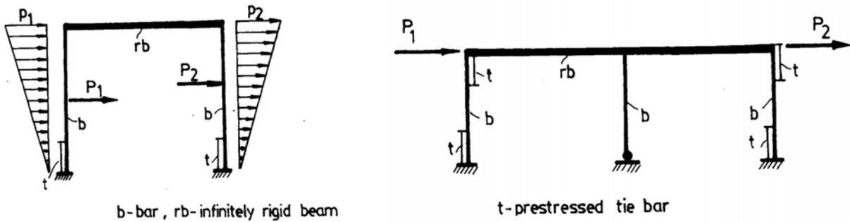
Fig. 1 – Examples of Prestressed Frames with the Infinitely Rigid Beam
