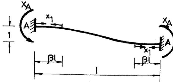
Fig. 5 – Deformed Axis of Prestressed Bar at Both Ends
