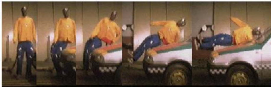
Figure 12 Sub-phases of the primary impact at 0, 50, 100, 150 and 200 ms, test 1 – pedestrian walking (see online version for colours)
