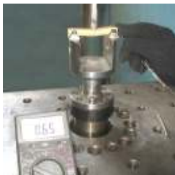
Figure 9: Checking on the stand, of the specimen temperature, using an electronic thermometer
