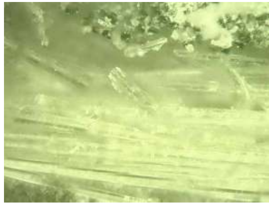
Figure 5 Specimen 3b Roving on weft magnified 500 times by 2D microscope
