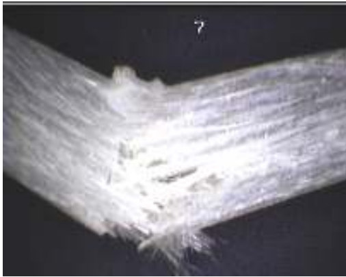
Figure 12 Specimen 8 MAT-Roving magnified 5 times by video camera
