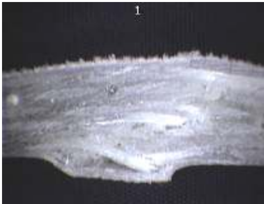
Figure 6 Specimen b4 Roving on weft magnified 5 times by video camera
