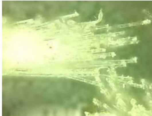
Figure 13 Specimen 5 MAT-Roving increased 500 times by 2D microscope
