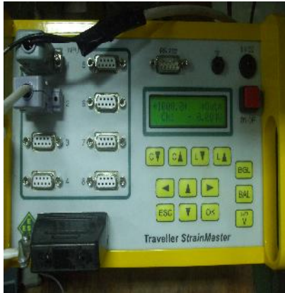
Figure 7: Strain gauge bridge Traveller StrainMaster
