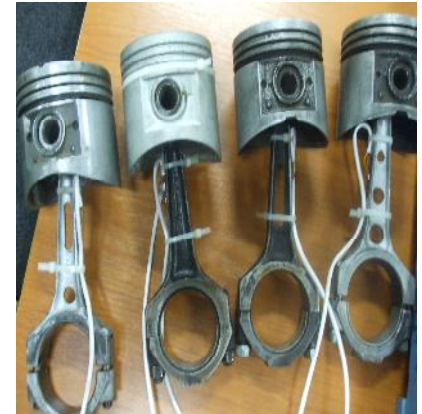
Figure 9: Different models for Con rod and piston tested
