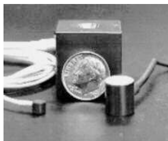
Fig. 4 Acoustic emission sensor [6]
