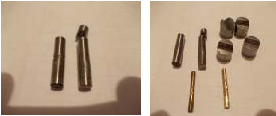
Figure 6: Scuffed pins and vee-blocks
