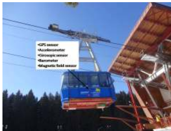
Figure 2: Arrangement of the sensors on the cabin [4]
