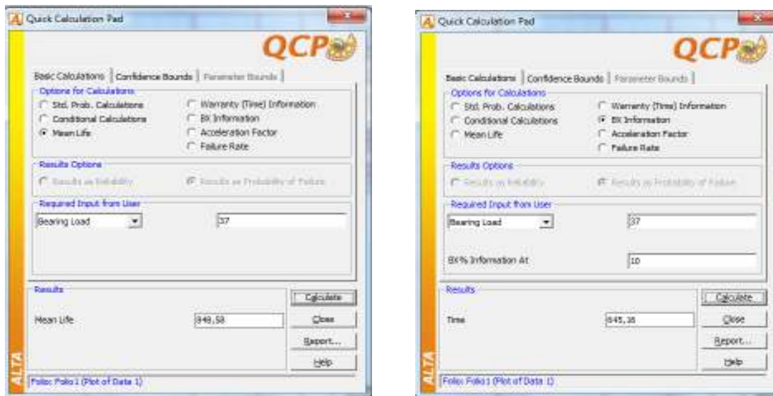
Figure 5: Reliability indicators of roller bearings type NN3020 a) Mean life b) B10 life
