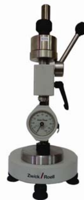
Fig. 2. The Shore hardness tester [4]
