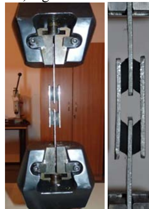
Fig. 8. The shear test of elastomer [7]
