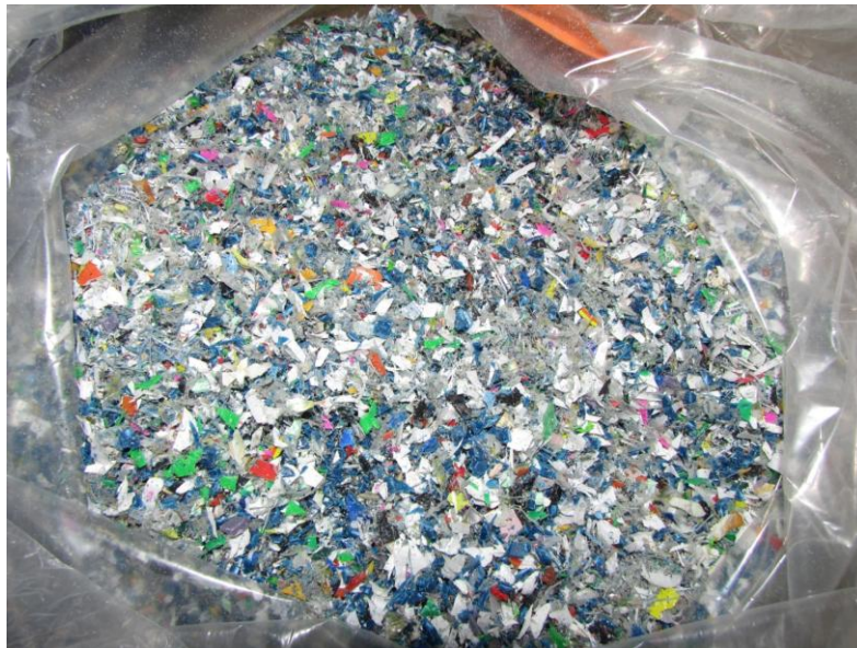
Figure 2. Cut and dried prepared plastic waste.
