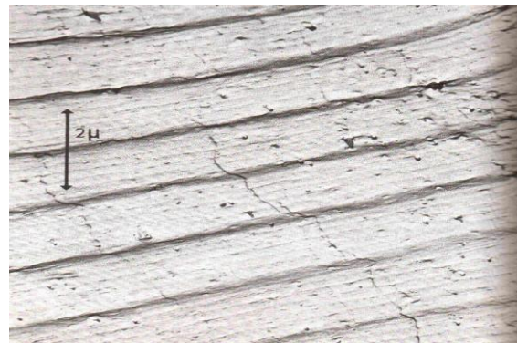
Figure 1b: The fatigue crack propagation front
