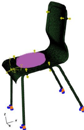
Figure 4: Loading scheme for the numerical model of the chair
