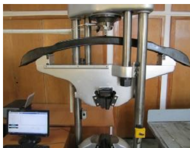
Figure 11: Bending test for steel car bumper shock absorber [1]
