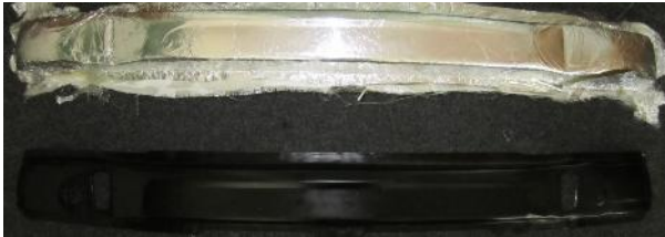
Figure 4: Bumper shock absorber made of composite materials removed from the mold [1]
