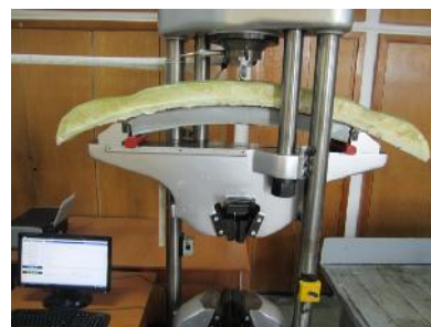
Figure 12: Bending test for composite car bumper shock absorber [1]
