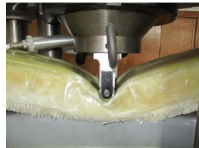
Figure 14: Bending detail for composite car bumper shock absorber [1]
