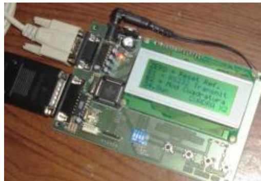
Figure 5: The hardware interface for signals decoding and measured values displaying, associated to the incremental displacement transducer
