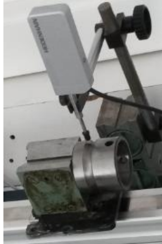
Figure 4: Example of dimensional measuring device arrangement for 3-D scanning and dimensional measuring of components with applications in automobiles field
