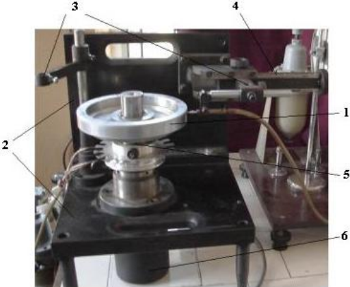
Figure 1: The manual shafts testing gauge, initial stage: 1- tested shaft/flywheel; 2 – base support plates; 3 – disposing systems for measuring devices; 4 – guidance for measuring devices disposing systems; 5 – fastening and fixing systems for tested shafts; 6 – housing for shaft’s bearings
