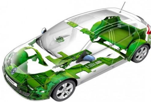
Figure 5. Parts in recyclable and renewable plastic material for Renault Megane vehicle
