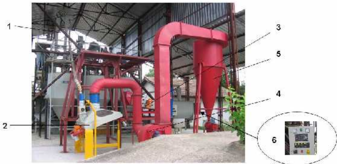
Figure.4. General view of of the installation used in experimental research 1 - elevator; 2 - gravimetric separator; 3 - intensive vacuum separator; 4 - fan, 5 - dedusting cyclone; 6 - control and signaling panel
