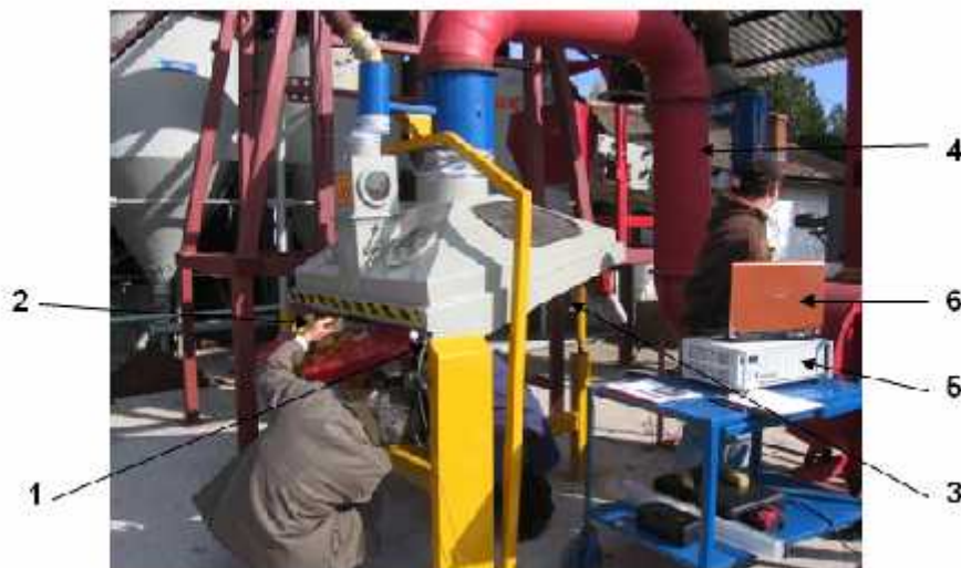
Figure 8. The location mode of measuring devices and adjustment areas 1 - displacement transducer; 2 - counterweights of vibrator; 3 – mechanism with screw; 4 - suction pipe; 5 - amplification and data acquisition module; 6 - laptop
