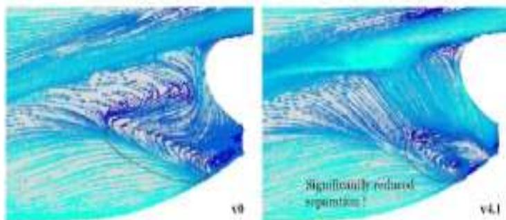
**Figure 5:** Limit streamlines on stern surface- FLUENT 6.3
