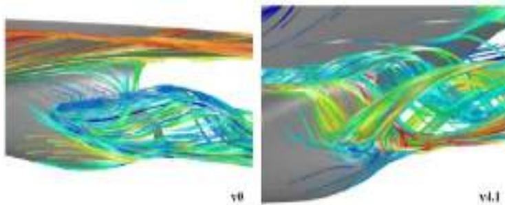
**Figure 4:** Vortex initiation and separation – FLUENT 6.3
