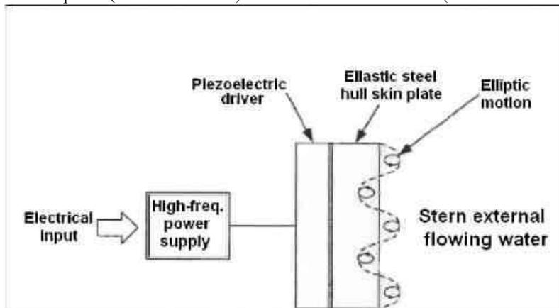
**Figure 6 :** Principle scheme of an ultrasonic vibrator
