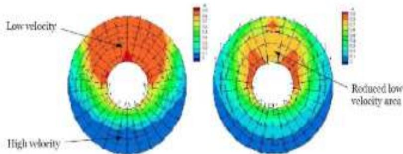
**Figure 2:** Comparison between experimental wake obtained for the model with initial stern shape design (left) and for the model with modified stern shape in conformity with the new concept design (right).
