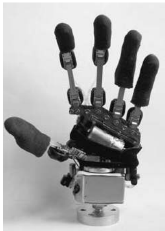
Figure 4 – The end-effector created for robot ARMAR
