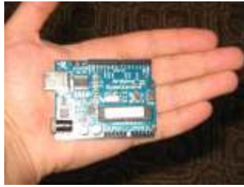
Figure 9 – The Arduino Duemilanove board [12]
