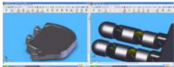
Figure 6 – The palm (left) and finger construction (right)
