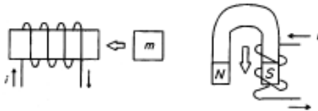
a) Maxwell electromagnetic force b) Lorentz electrodynamic force
