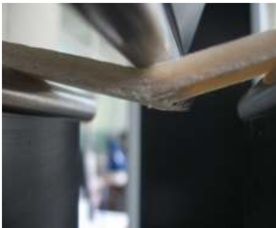
Figure 1: Experimental 3-point bending configuration and composite sample positioning
