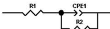
Fig.1 Equivalent circuit which schematically describes the electrochemical behavior of Ni/Si 3 N 4 -SiC, Ni/ TiO 2 and Ni/CNT coatings
