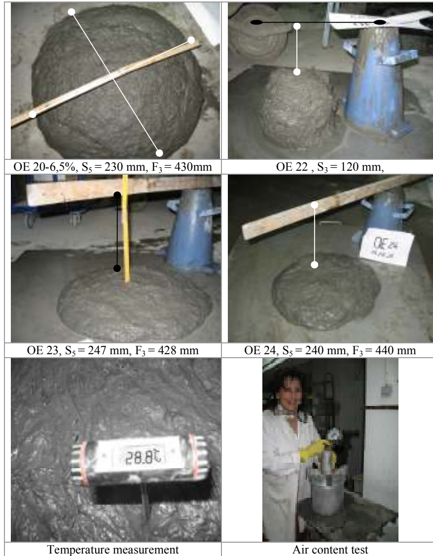
Figure 3: Fresh mix properties testing
