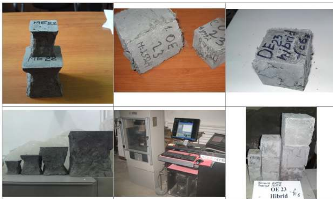
Figure 4: Specimens after the 6th day test (cubes with the edge of 50 mm, 70.1 mm, 100 mm and 150 mm)
