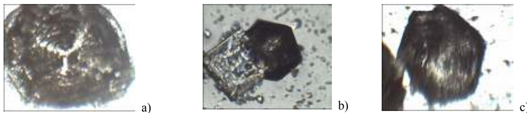
Fig. 5: Crystalline structures found out in the three parts of ASP solutions (a-middle, b - upper, c – lower)
