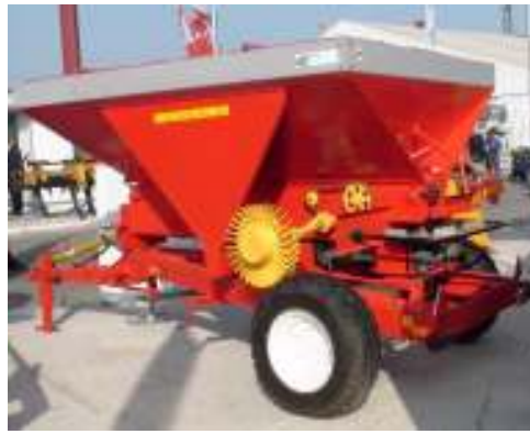
Figure 1: The machine of applying chemical solid fertilizers, MA 3.6 a) front perspective view b) rear perspective view
