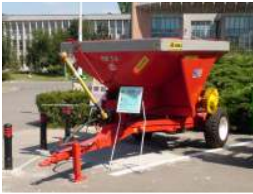
Figure 1: The machine of applying chemical solid fertilizers, MA 3.6 a) front perspective view b) rear perspective view
