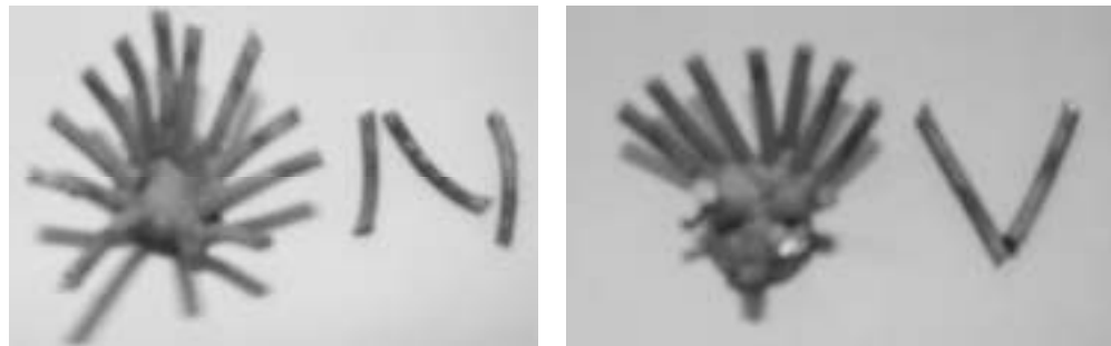
a) Co-Cr alloy b) Ni-Cr alloy Figure 2: Dental alloy sprue base and sprue pins, after cast or re-cast process
