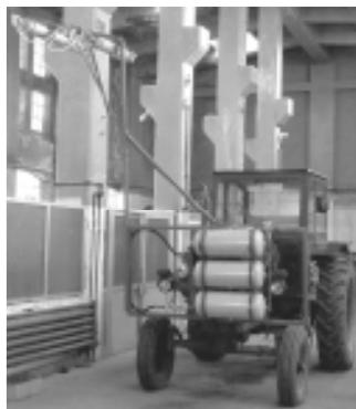
Figure 1: Modular equipment for nuts harvest by pneumatic impulses
